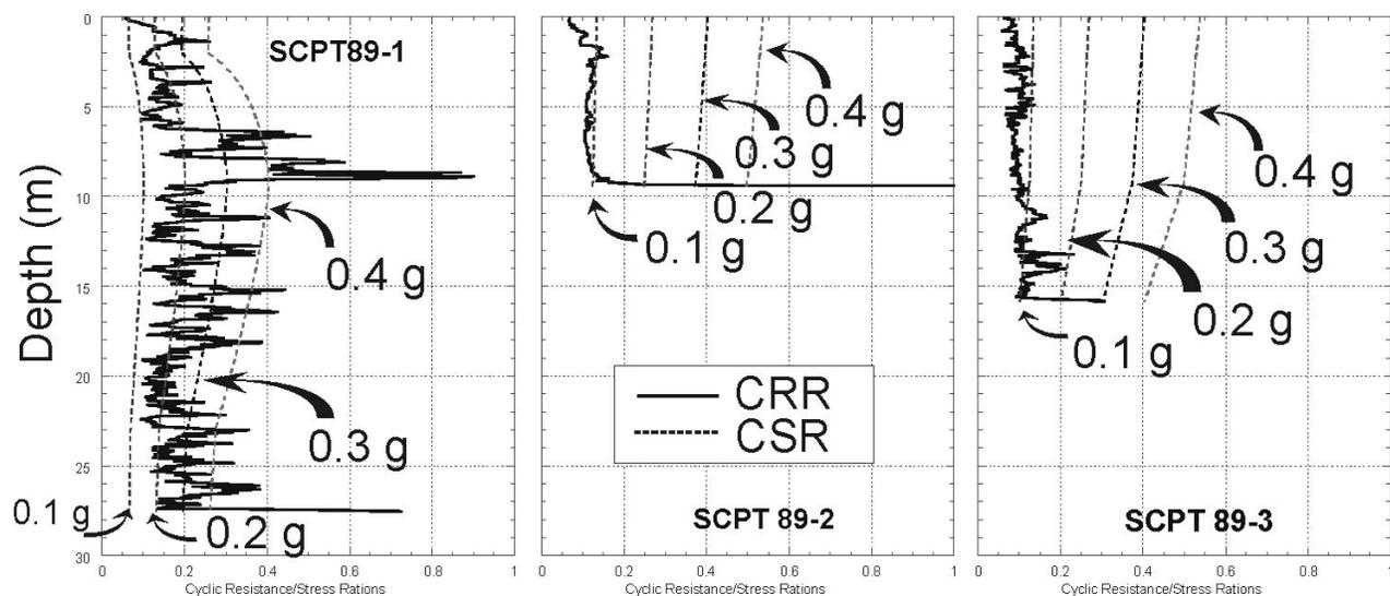
Figure 8. Cyclic resistance ratio (CRR) and cyclic stress ratio (CSR) plots of sites 89-1, 89-2 and 89-3 based on the CPT data. Where CRR values are less than CSR values the Factor of Safety exceeds 1 and liquefaction is likely.
