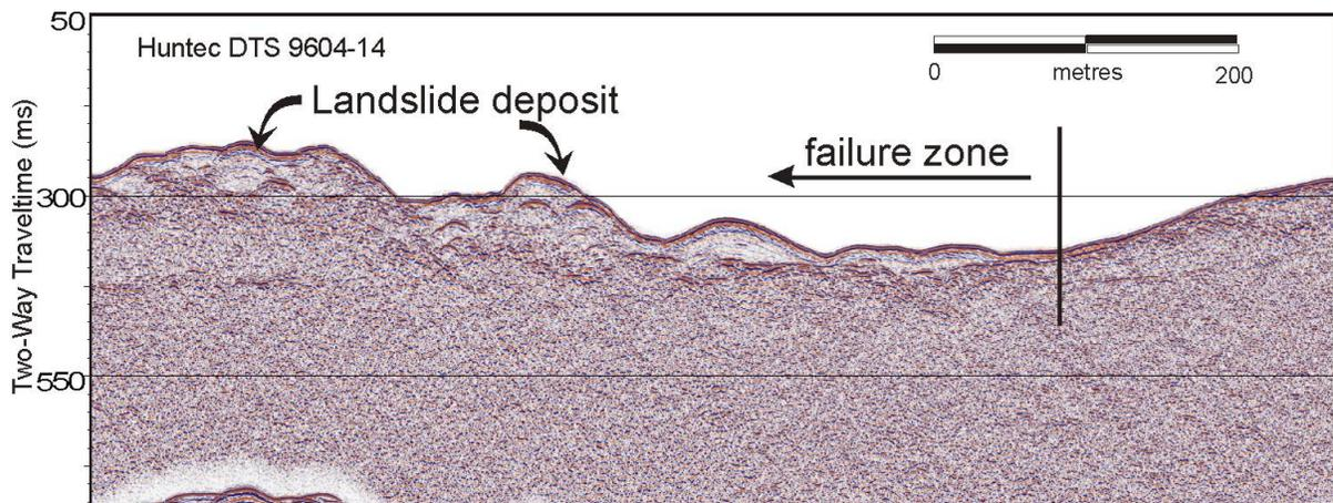
Figure 10. Hunttec boomer seismic reflection profile across the Grief Point submarine landslide.
