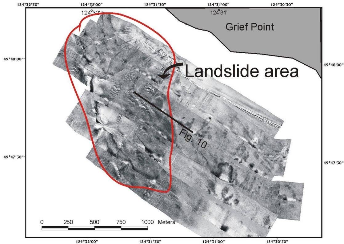
Figure 9. Sidescan sonar mosaic of the Grief Point landslide. Water depths span from 20 m in the north to 220 m in the southwest area of the image. The location of a seismic section (Fig. 10) is shown.
