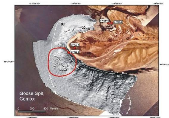
Figure 5. Artificial Sun-shaded multibeam bathymetry and airphoto of Goose Spit. The dots represent Cone Penetration Test (CPT) holes, the data of which are used in this study. The area within the broad circular outline is what is believed to be the landslide deposit resulting from the 1946 earthquake.
