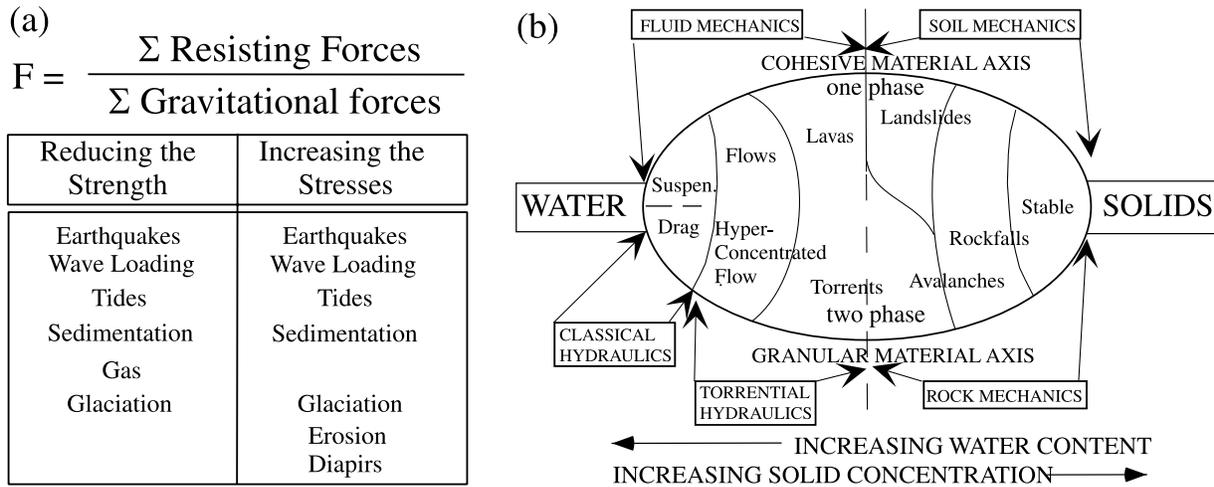
**Fig. 2.** Classification of submarine mass movements adapted from subaerial classification proposed by the ISSMGE Technical Committee on Landslides (TC-11).
